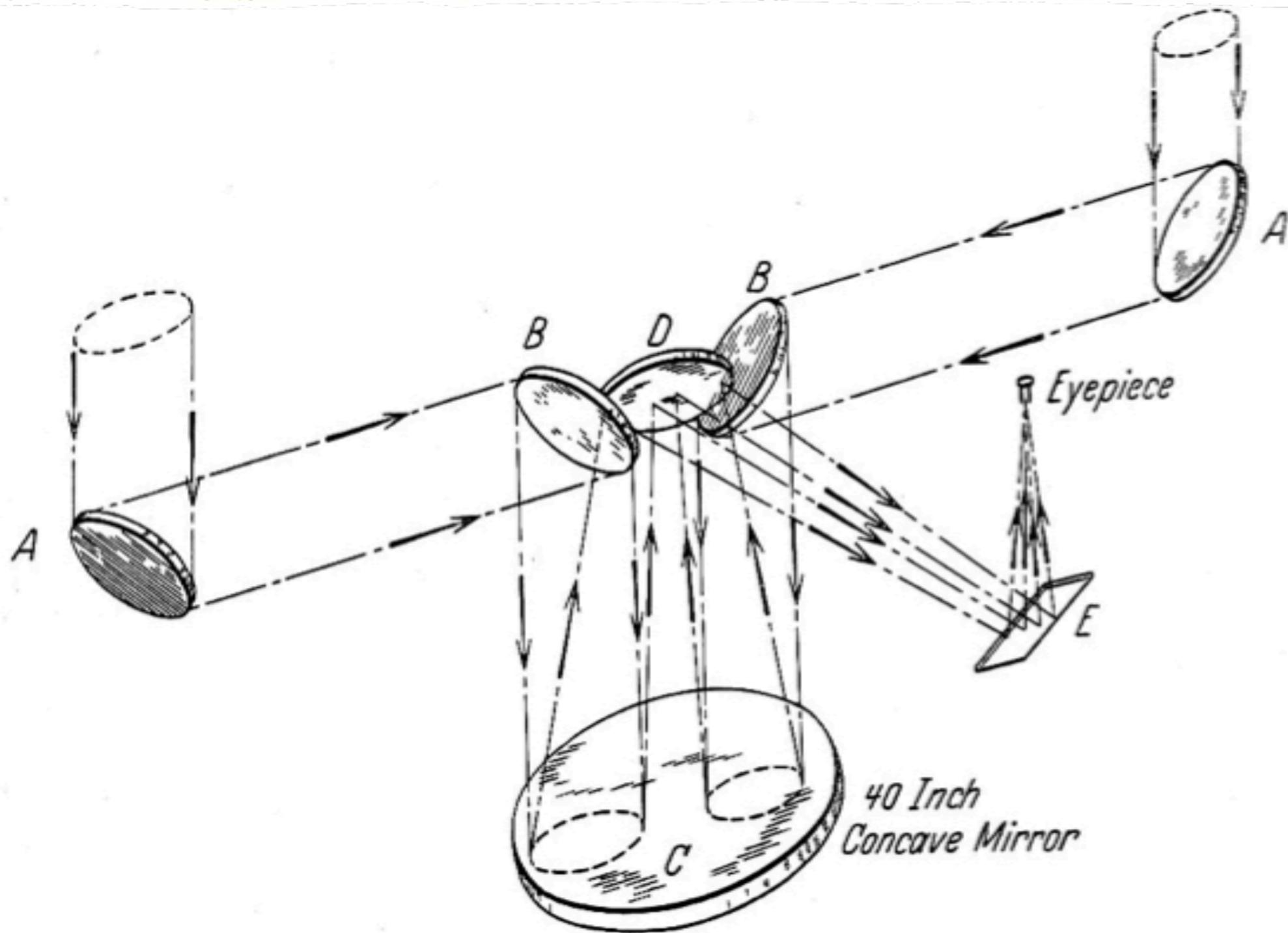
Abb. 8. Diagram of light path in 50 foot interferometer.
