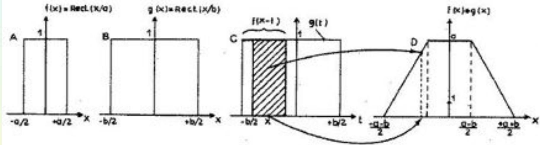
Convolution product of two 1D rectangle functions. A)  $f(x)$ , B)  $g(x)$ , C)  $g(t)$  and  $f(x-t)$ ; the dashed area represents the integral of the product of  $f(x-t)$  and  $g(t)$  for the given  $x$  offset, D)  $f(x)*g(x) = (f*g)(x)$  represents the previous integral as a function of  $x$ .
