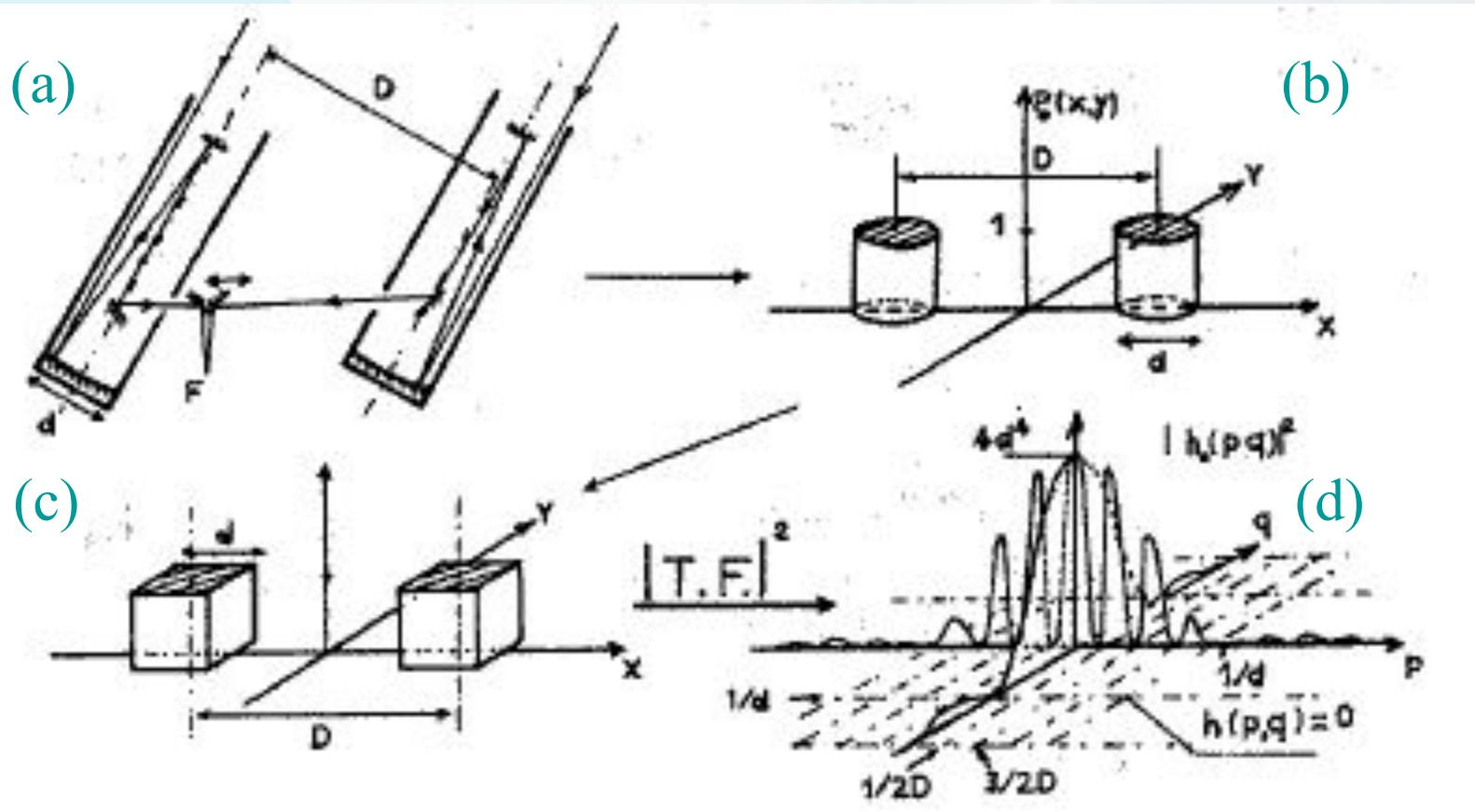
Two coupled optical telescopes: simplified optical scheme (a). Distribution of the complex amplitude for the case of two circular (b) or square (c) apertures and corresponding impulse response (d).
