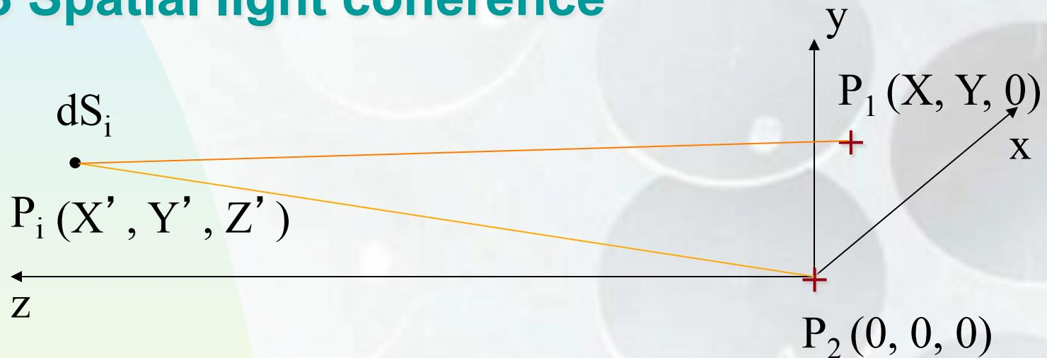
$$|r_2 - r_1| = |P_2 P_i - P_1 P_i| = |-(X^2 + Y^2) / 2 Z' + (X \zeta + Y \eta)| \quad (5.3.9)$$
